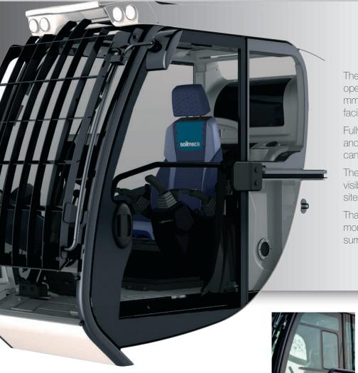
The ergonomic H-cab model embraces the operator. A unique solution in this category (1050 mm /41.6 in wide) in which several accessories facilitate the work of the operator.
